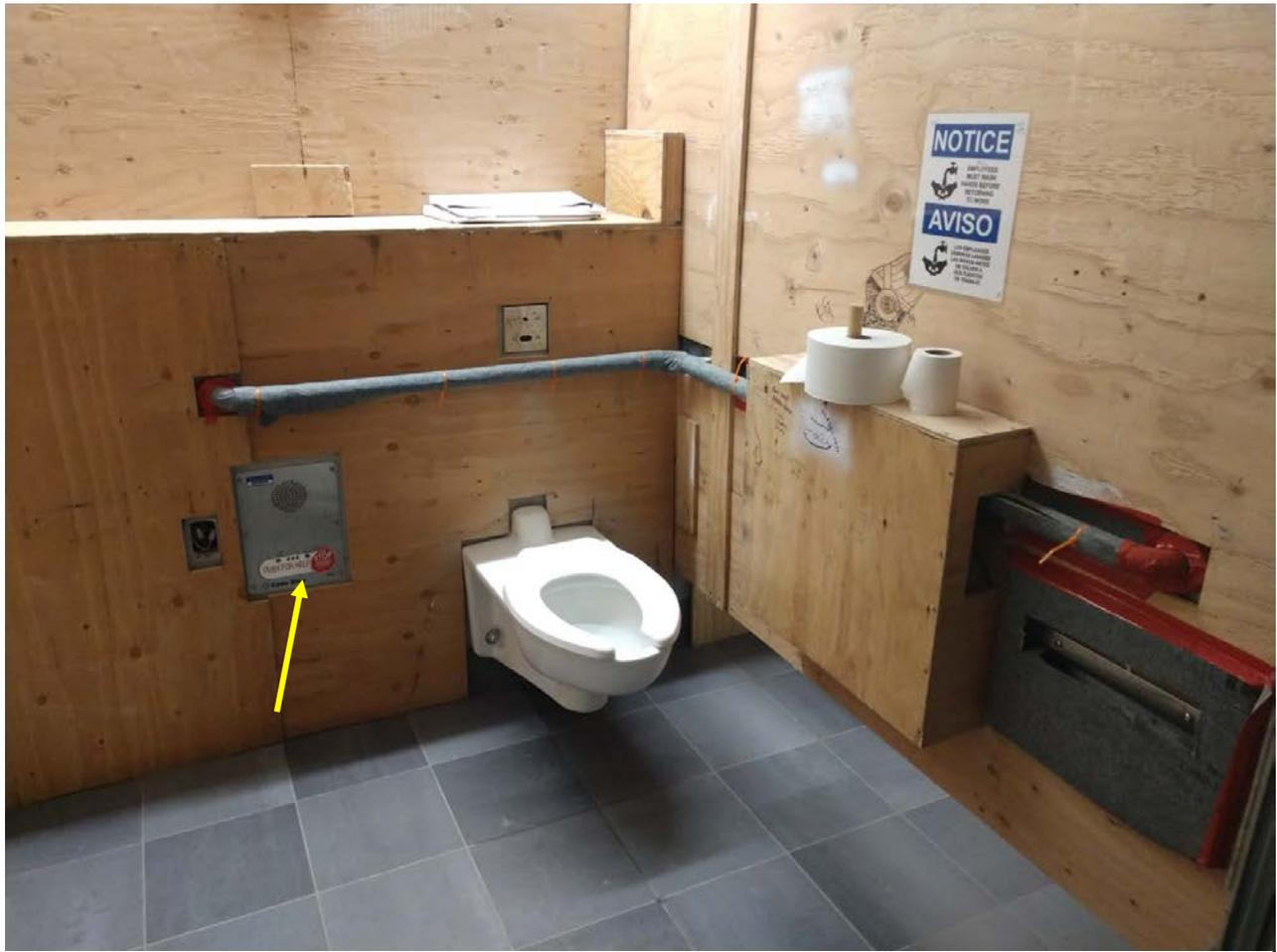
Pictured above is the accessible stall in one of the restrooms. The walls are covered by wood. A grab bar is visible above the toilet. To the left is a panic box with button for emergency calls if needed.
